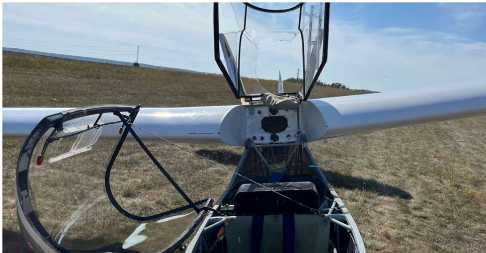
Fig. 1 – Damaged rear sailplane canopy
